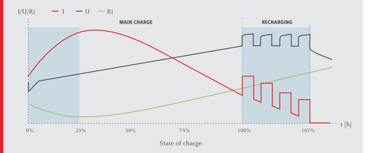
losses when charging commences and during the recharging phase. The battery only receives the current that it life to its maximum. actually needs.
